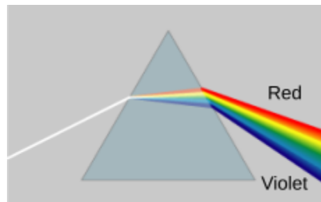
Figure 1. Dispersion via a Simple Prism. This diagram shows a basic prism leading to the dispersion of light—splitting white light into its different components. Source: Wikimedia Commons
