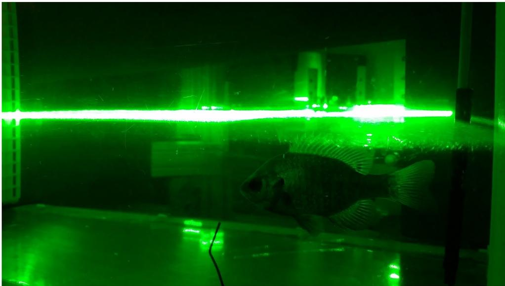
**Figure 1. Side View of a PIV Experiment.** When this fish swims in the light sheet at the center of the screen, scientists can film its movements with a high speed camera below the tank. By tracking the particles in the water, scientists can visualize and measure how water is moving around the swimming animal.
