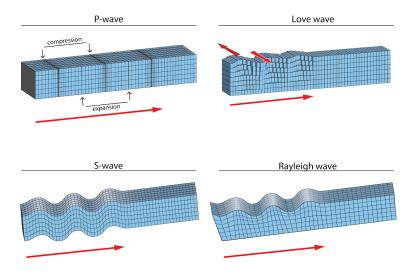
**Figure 1. The Four Main Types of Seismic Waves.** Two types of seismic waves, s-waves and p-waves, travel through Earth while Love waves and Rayleigh waves travel along Earth's surface. S-waves and p-waves travel faster than Love and Rayleigh waves, but Love and Rayleigh waves tend to do the most damage to structures.
